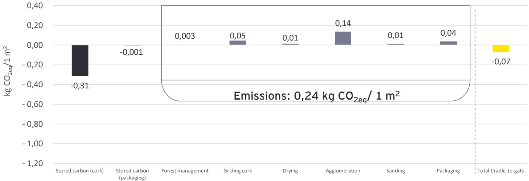
**56%** emissions associated with agglomeration process, **19%** emissions associated with grinding process
