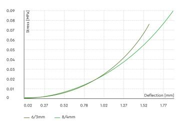
Note: Following ISO8013-1998 measured in Cantilever Test System
