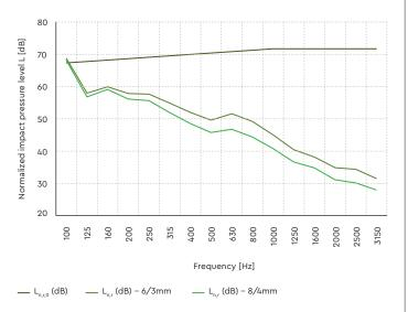
Normalized impact sound pressure level of the reference floor L<sub>n,r</sub> with the floor covering under test
