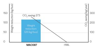
(a) comparing against a HML core (2500 kg/m³), in a configuration 6/3/6 an 500kg/m³ plywood
