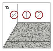
Never mechanically fasten the underscreed or the pre-attached foil barrier with screws, nails or staples as this will severely diminish the performance of the insulation barrier.
