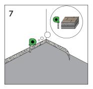
Install a perimeter insulation barrier vertically around the entire perimeter of the room with width equal to that of the floor build up.
