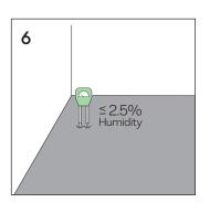
The humidity content of the subfloor is critical: it must not exceed 2.5 % (MC).
