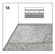
Cast a suitable screed over PE foil.
