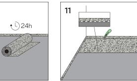
Cut and trim the underscreed to the designed size to fit the installation. Apply directly over the slab. In case of profile material, dimple side must face down.
