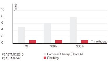
**TD 7000** sealing material is compounded with Silicone (VMQ) rubber. This product is recommended for most transformer oils with an outstanding resistance to extreme temperatures.
