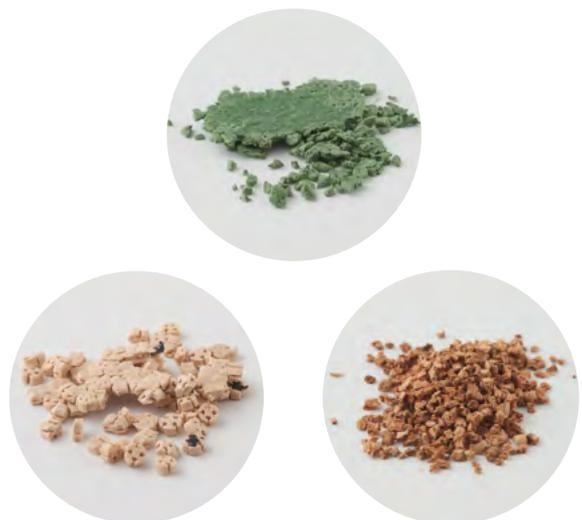
EPDM, TPE e Cork infill after an assay of 1 hour at 65°C and 2N/mm<sup>2</sup>
