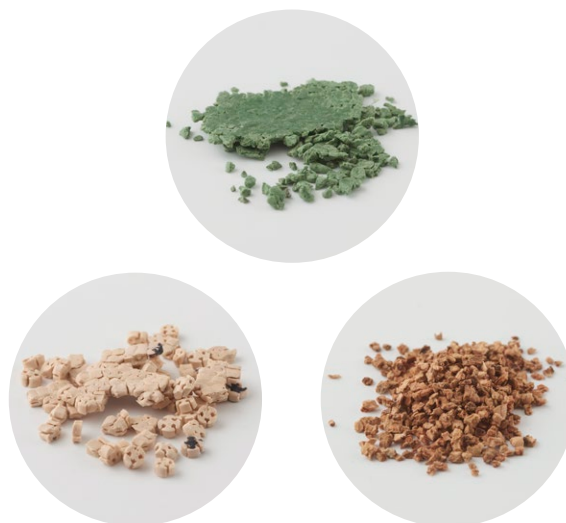
EPDM, TPE e Cork infill after an assay of 1 hour at 65°C and 2N/mm 2
