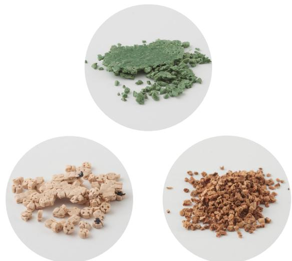
EPDM, TPE e Cork infill after an assay of 1 hour at 65°C and 2N/mm²
