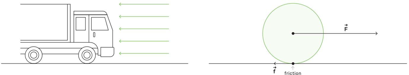
Another example is the resistance faced by a car. The resistance is the result of the rolling friction of its tyres and the air resistance.
