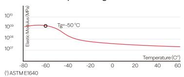
TD 1310 sealing material is compounded with special Nitrile (NBR) rubber. This product is recommended for most transformer oils with an outstanding resistance to low temperatures.
