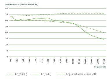
$L_{n,r,0}$  – Normalized impact sound pressure level of the Lab reference floor.
