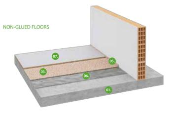
01. Reinforced concrete slab
