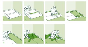
1. Installation of the moisture barrier; 2. Installation of the tape on the seams ; 3. Installation of perimeter barrier; 4. Installation of underlay; 5. Installation of the tape on joints between rolls; 6. Installation of final flooring; 7. Cutting perimeter barrier.
