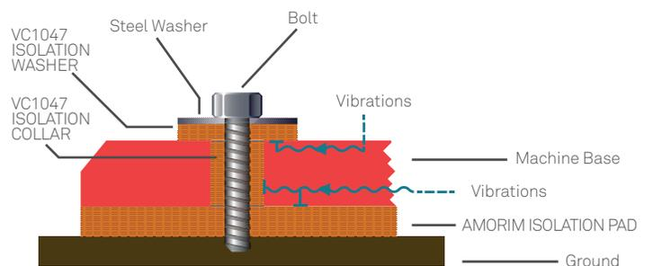
The main principle in **FIGURE 2** should be encompassed whenever using isolation pads. The basic principle is to provide isolation between the source of the vibration and any part of the system that can transmit the undesired sound.
