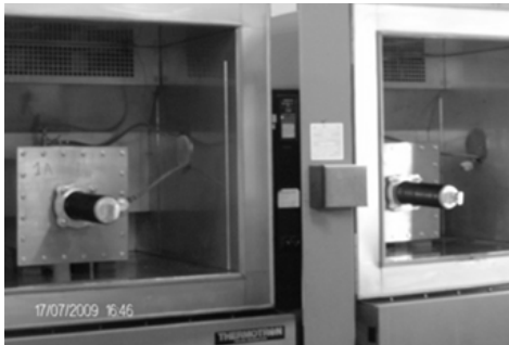
Thermal cycle of +5°C for 8h to 110°C for 14h; 14 days
